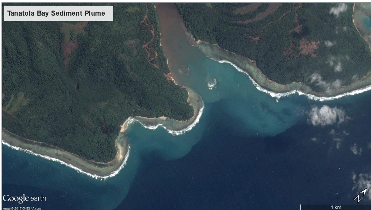
Figure 7: Aerial photograph showing increased sediment concentrations in the receiving waters from freshwater sources (imagery date 7 July 2013).
