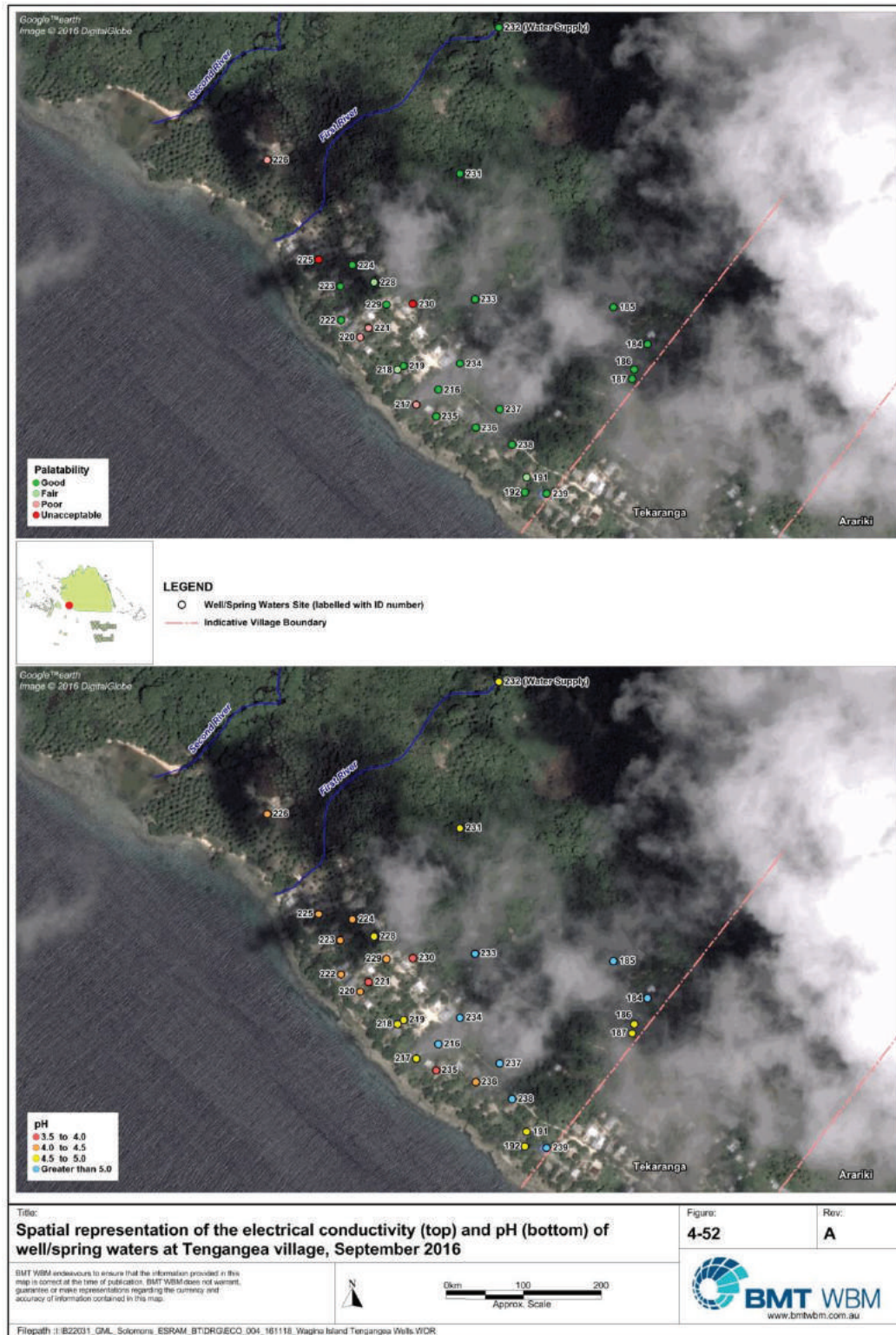
Figure C-5 Spatial representation of the electrical conductivity (top) and pH (bottom) of well/spring waters at Tengangea village, September 2016
