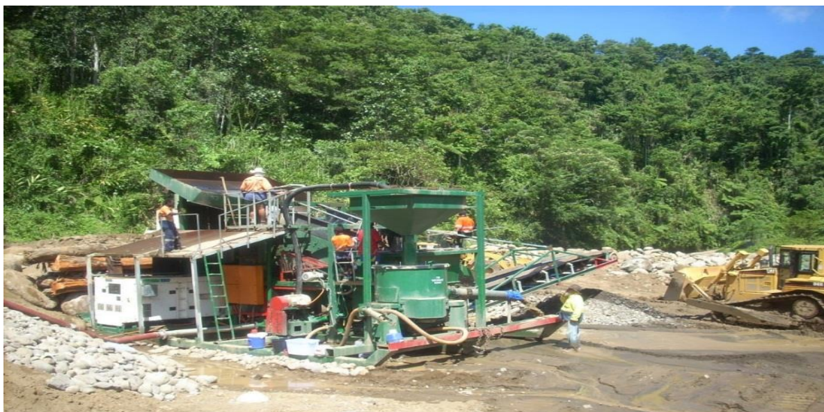
Figure 13: SAMs plant for processing river gravels.
